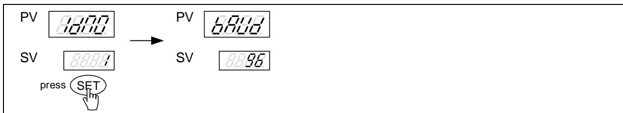
10. Press SHIFT key then lower display will start flash, press UP key or DOWN key to select baud rate then pressing SET key to save the current setting.
