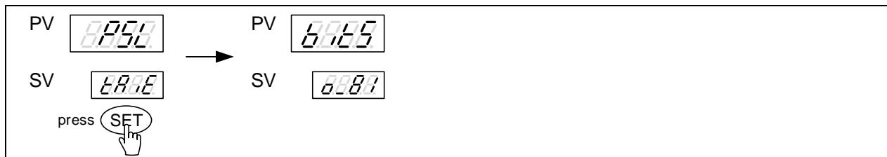
6. Press SHIFT key then lower display will start flash, press UP key or DOWN key to select DATA format then pressing SET key to save the current setting.
