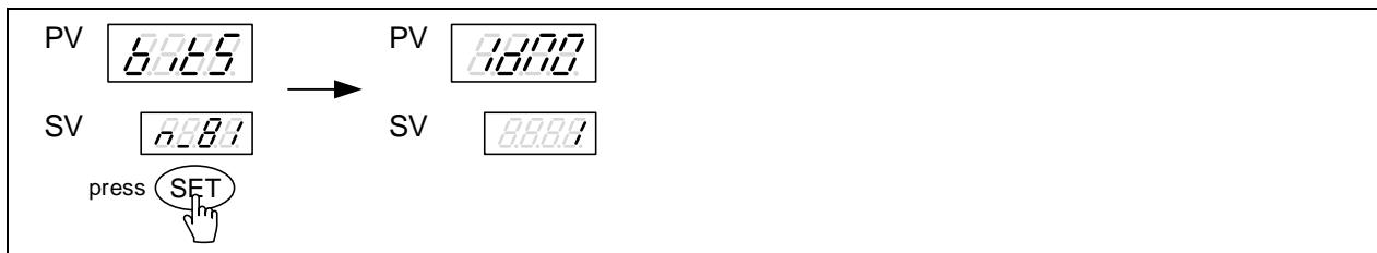
8. Press SHIFT key then lower display will start flash, press UP key or DOWN key to select slave address then pressing SET key to save the current setting.
